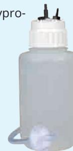
2l borosilicate glass collection bottle with high chemical resistance, with splinter-proof coating, special bottle head for minimized foam and aerosol formation, hose nozzle for VacuuHandControl VHC<sup>pro</sup> and additional port to connect a second VHC<sup>pro</sup> (optional), hydrophobic filter element 0.2 µm to protect pump and environment, hose for connection to pump unit BVC or BVC basic; fully autoclavable.
